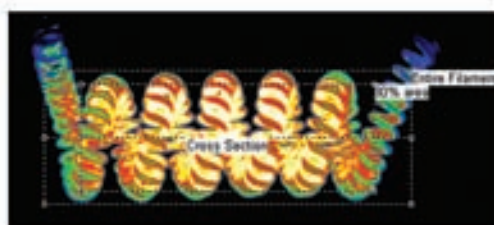
Evaluation of a luminance distribution of a filament (LMK - filament, logarithmic representation)
