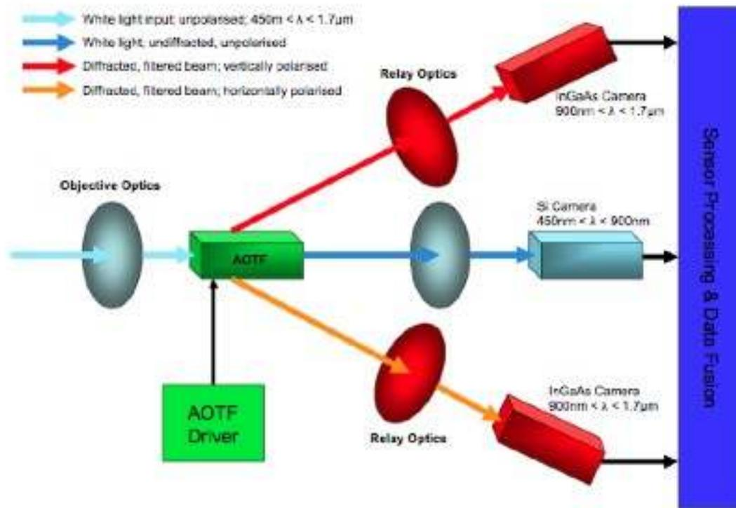
Figure 1 Schematic of polarimetric hyper-spectral imaging system
