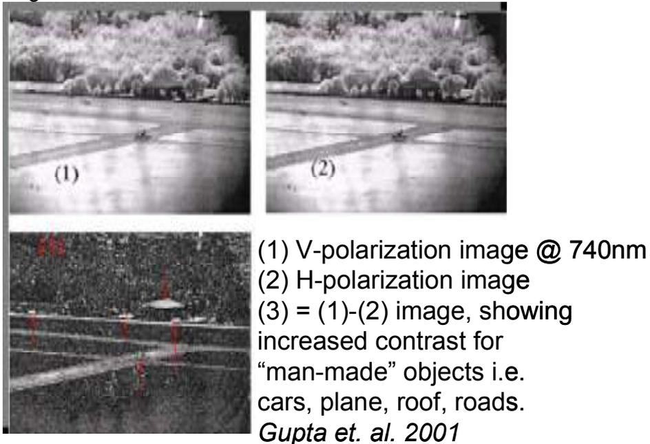
Figure 5 Enhancement of detection by differential polarisation imaging
