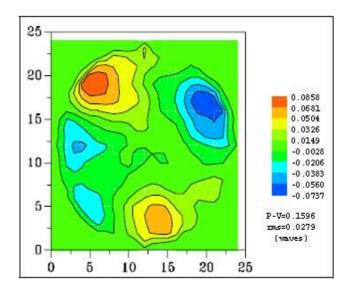
The 3D and contour plot shows the presence of astigmatism both for Zygo and for Optino. The contour plot shows the good agreement between Zygo and Optino.
